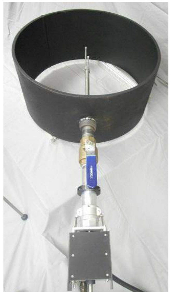
Motorized SwivelSampler mounted on demonstration coal pipe
