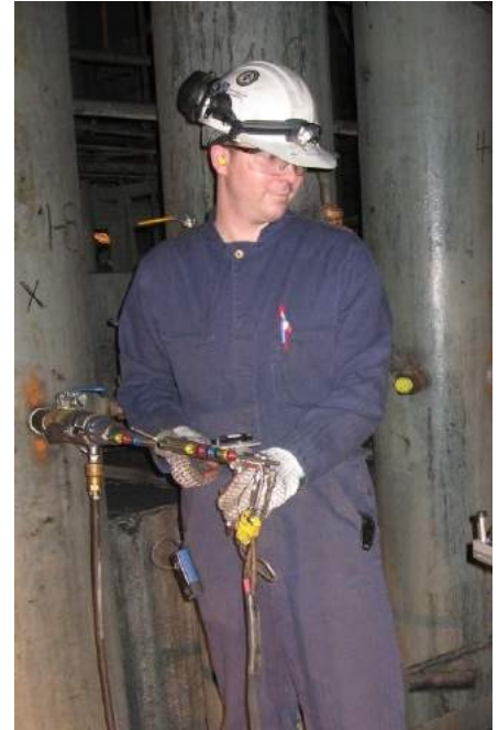
Velocity testing in a coal piping system
