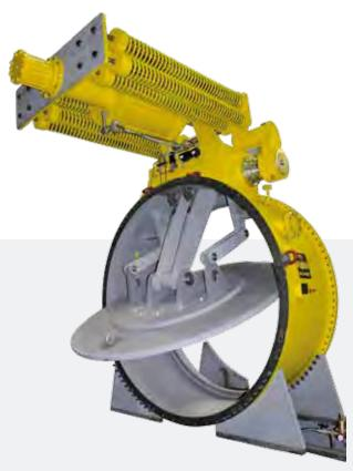
KÜHME valves are used in steelworks in order to quickly and safely shut off blast furnace gas, converter gas and coke-oven gas. The valves are capable of withstanding exceptional conditions and function reliably, for example, even at temperatures up to 280 °C and with a high ratio of dust.
